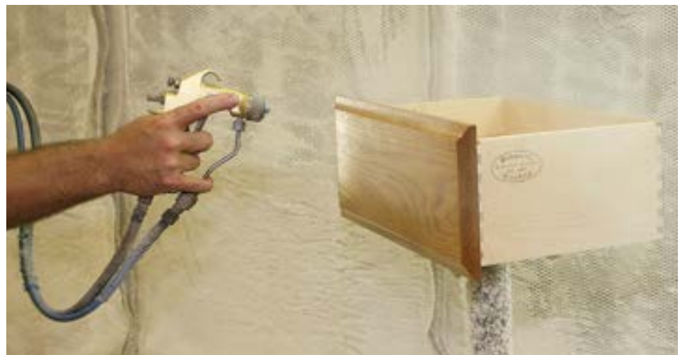
The sealer and top coat are carefully applied, giving each piece a smooth and durable finish.
