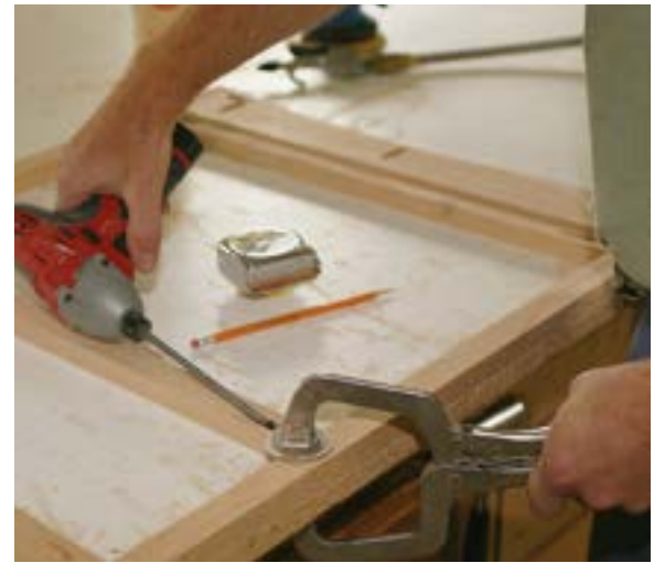
Face frames are precisely measured and assembled with pocket screws.
